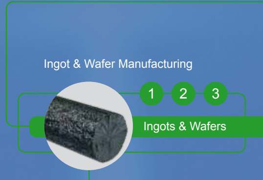
Fig. 3 : Monocrystalline Silicon (Czochralski Process)
