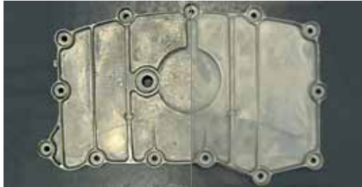
Visual comparison of a conventional vacuum process (left hand) with Vacu 2 from Pfeiffer Vacuum (right hand) following glow test at 500 °C
