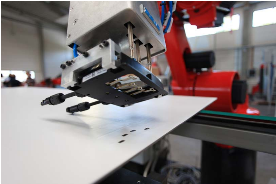
Placing of the J-Box
